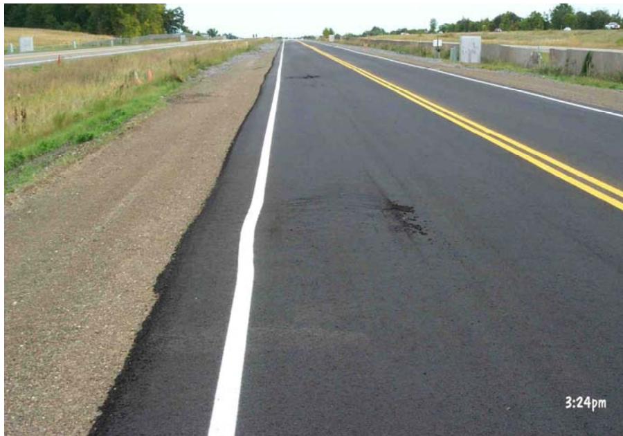
Figure 1.4- Oil Gravel after 38 Laps of the MnROAD Truck
