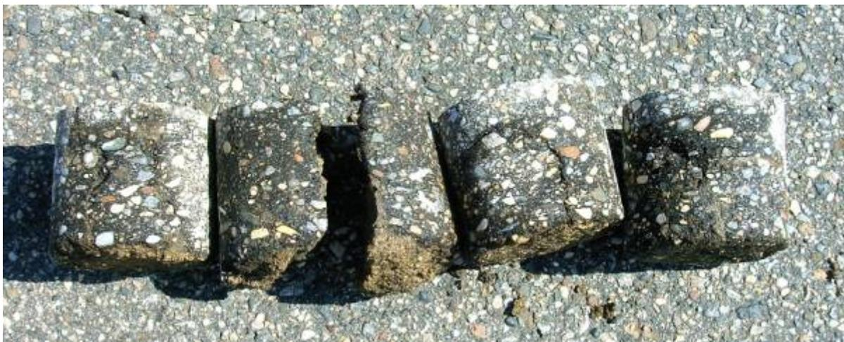
**Figure 3. Cores Showing Cell 1 Structural Integrity**
